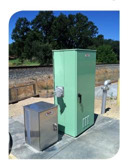
The TESCONNEX® Sump Termination Panel is a NEMA-type 3RX cable entry cabinet with two physically separate sections designed to isolate potentially hazardous or corrosive sewage gasses from electrical cable termination points and vent the gasses into atmosphere.
